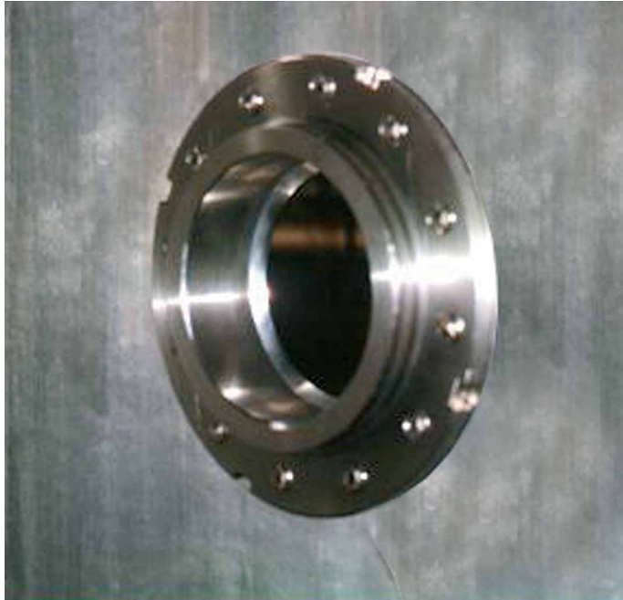
Figure 2: Adaptor seen from outside the tank
