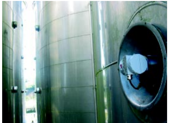
Figure 4: DT302S Installed on a Fermentation Tank
