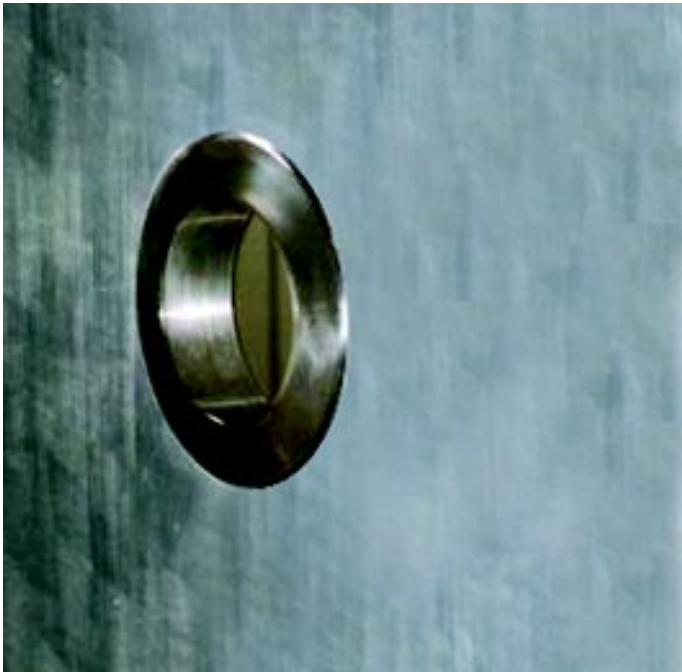
Figure 3: Adaptor seen from inside the tank
