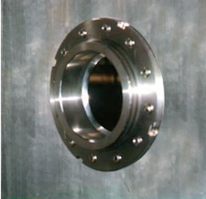
Figure 2: Adaptor seen from outside the tank
