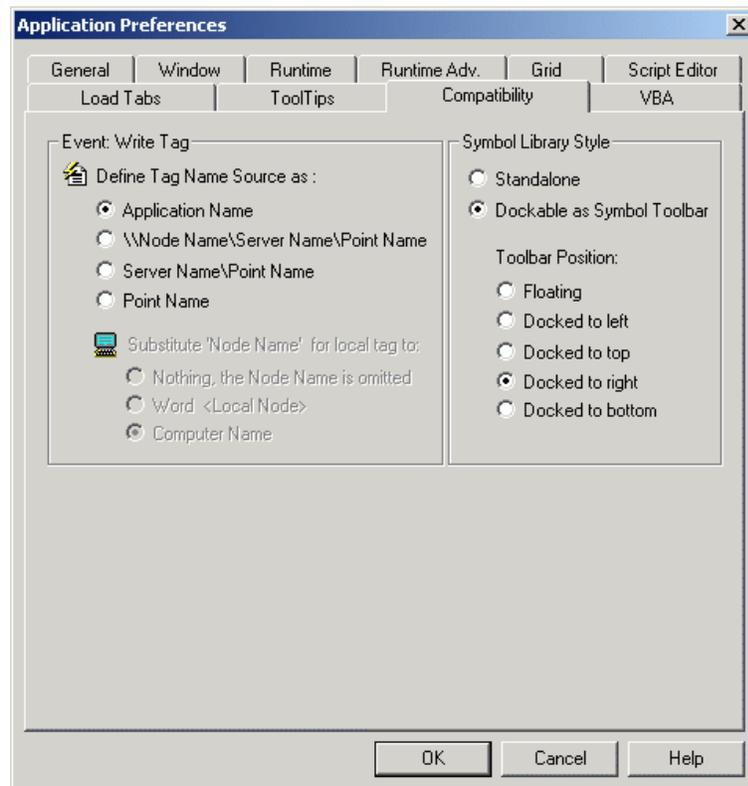
**Figure 24. Switching Between Stand-alone and Dockable Symbol Modes**
