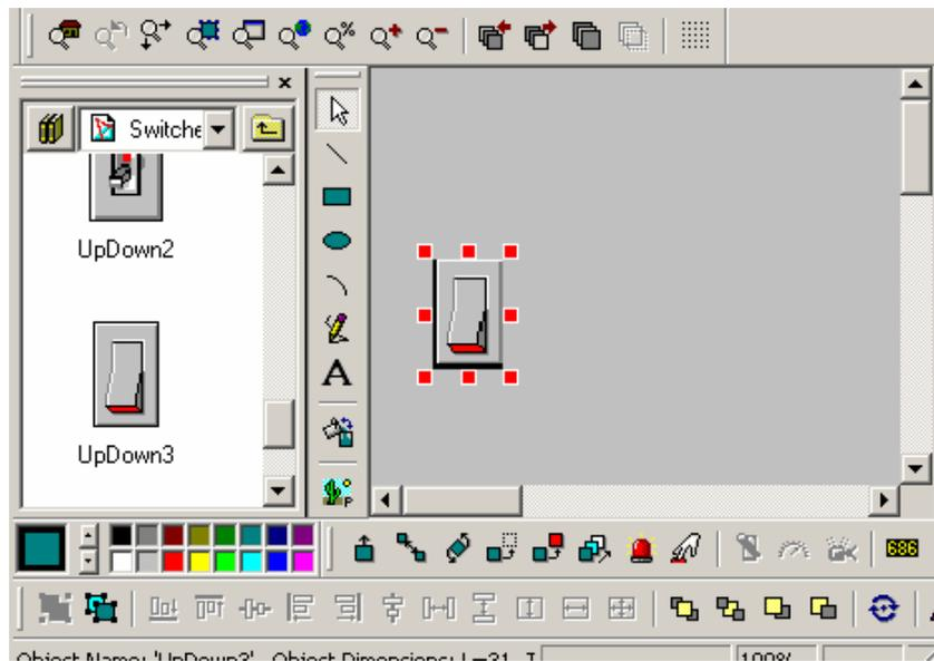
Figure 1. Switch Symbol in GraphWorX Display
