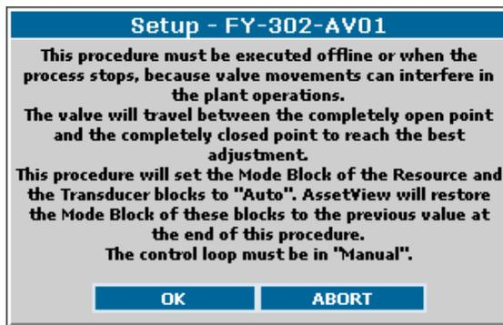
Figure 36. Configuring the Mode Block
