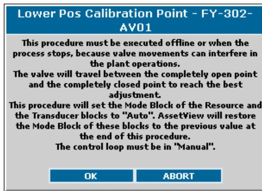
Figure 24. Configuring the Mode Block
