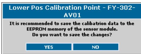
Figure 29. Saving Calibration Data
