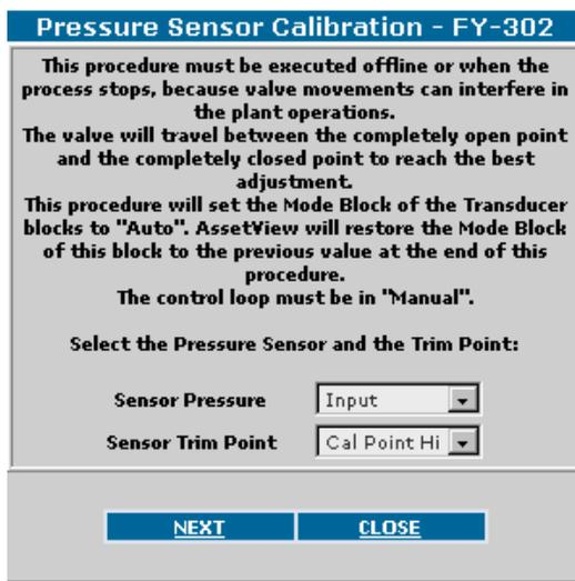
Figure 42. Checking the Sensor Pressure
