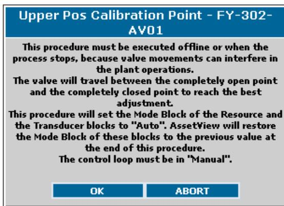
Figure 30. Configuring the Mode Block
