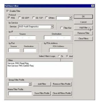
Figure 4.4. Creanting a Filter by Service
