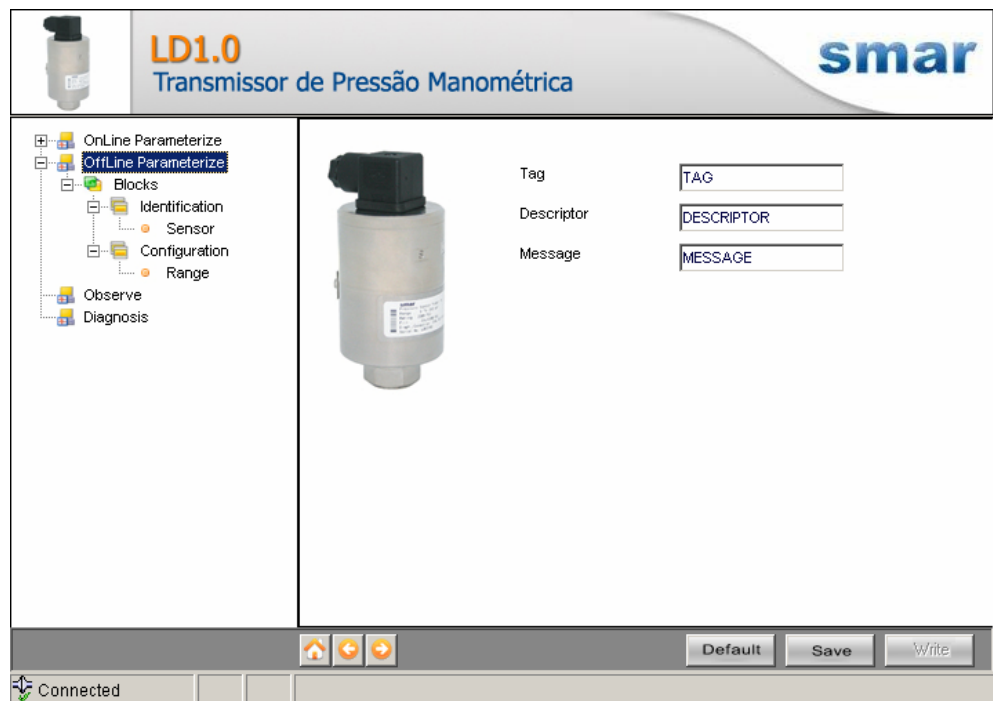
Figure 4 – LD1.0DTM “Offline Parameterize” Screen
