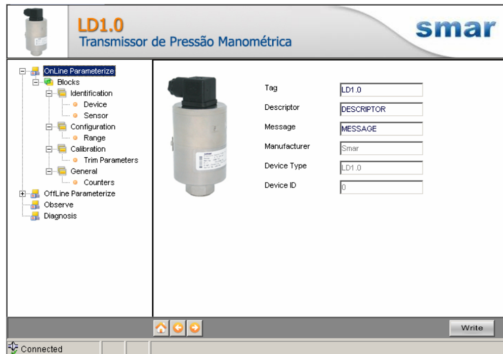
Figure 3 – LD1.0DTM “Online Parameterize” Screen
