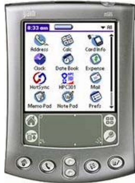
Figure 3.1 - Smar's HPC301 Hand-Held Terminal
