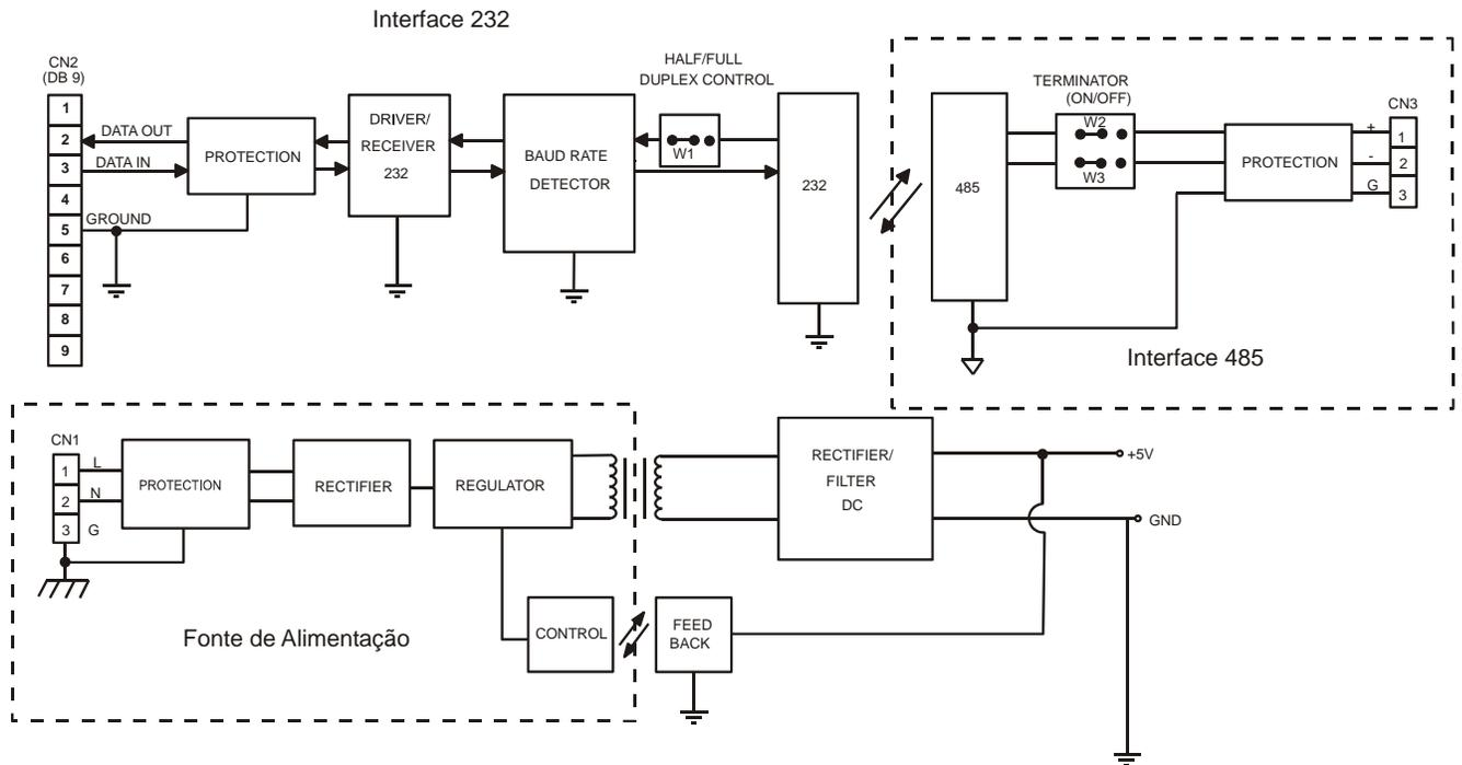
**Fig.1 – ICS2.0P Interface Block Diagram**
