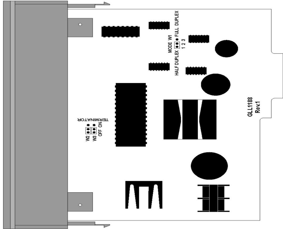
Fig. 2- Position of the Jumpers on the electronic board
