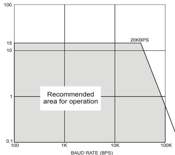
**Fig 11.- Recommendation for the EIA 232 standard (shielded cable, moderated EMI)**
