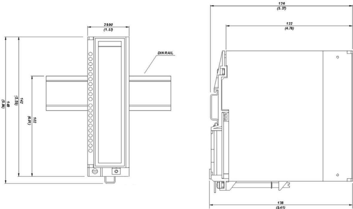
Fig. 7 Dimensional drawing of the ICS2.0P mounted in the DF9 support.
