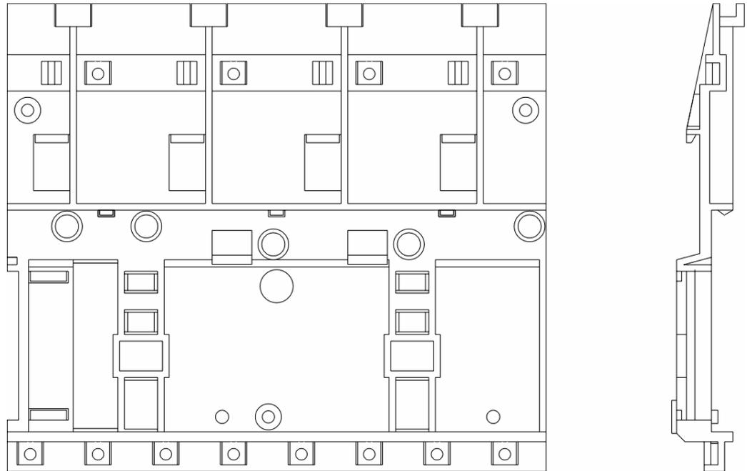
**Fig.7- Perspective drawing of the R-700-4 rack**
