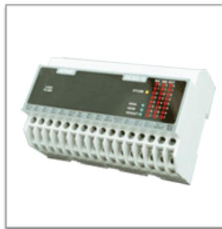
Discrete data is processed by a Flexible Function Block, that may be located on the CPU or even in a dedicated FFB located in the DC302 itself. In this case, a control cycle of 100msec is possible for local control and interlocks, while only integration data is published on H1 channel for integration with other devices. Logics are maintained even in the event of main CPU failure, as long as power is maintained, keeping full benefits of FF architecture.
