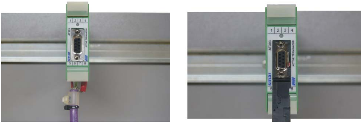
Figure 5 – AT303 on DIN rail with direct connection and using Profibus connector
