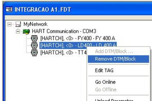
Figure 12. Removing a Device
