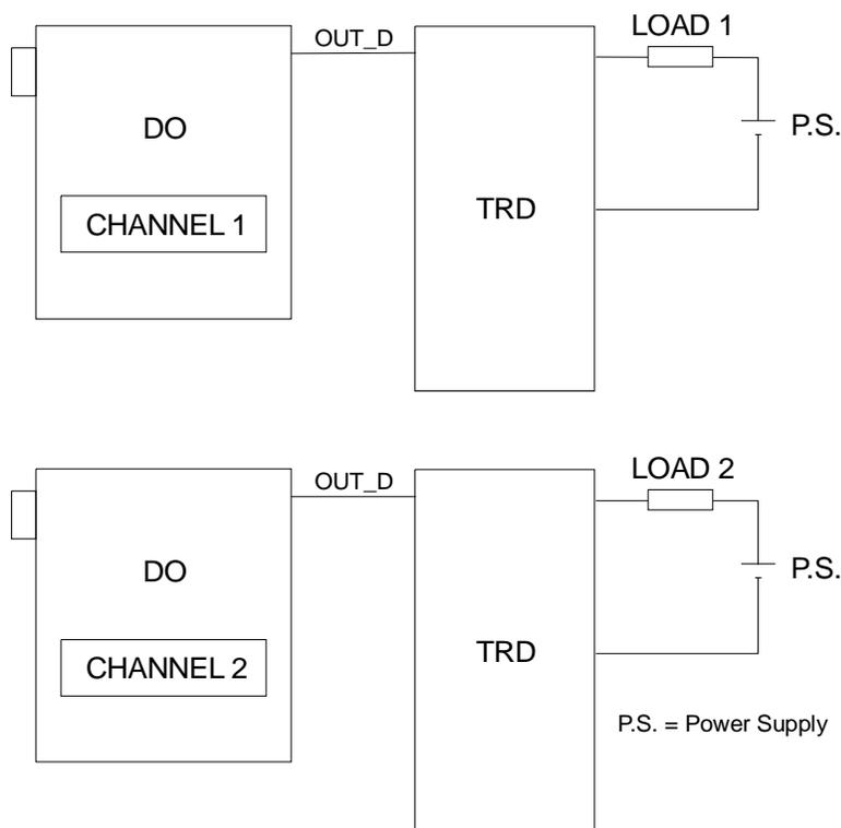
**Figure 3.2 - FR302 and DO Block connections**
