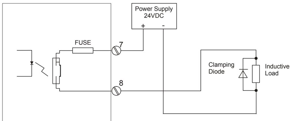
Figure 1.7 – Protection Diode in Parallel to DC Load
