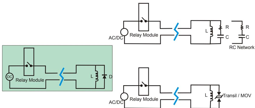
Figure 1.6 – Filters for AC and DC loads
