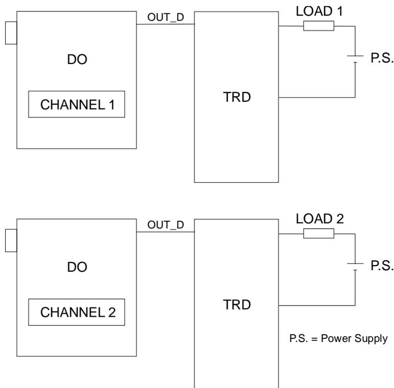
**Figure 3.2 - FRI302 and DO Block connections**
