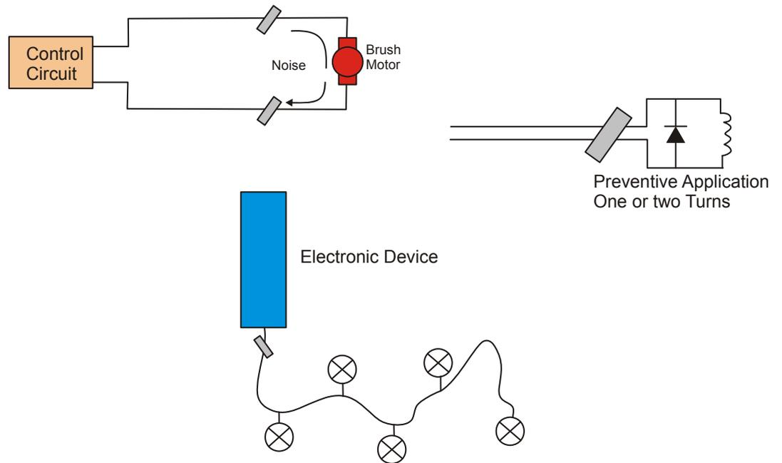
Figure 1.9 – Ferrite Application on Control Lines
