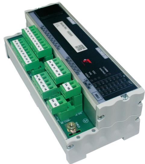
Discrete data is processed by a Flexible Function Block, that may be located on the CPU or even in a dedicated FFB located in the DC302 itself. In this case, a control cycle of 100 ms is possible for local control and interlocks, while only integration data is published on HI channel for integration with other devices. Logics are maintained even in the event of main CPU failure, as long as power is maintained, keeping full benefits of FF architecture.
