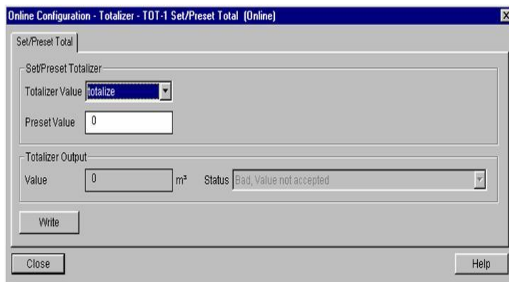
Figure 3.20 - Set/Preset Configuration for Totalizer Block - Simatic PDM
