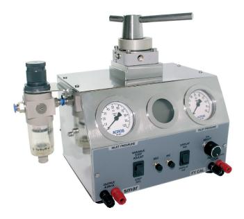
The FYCAL designed to calibrate the piezo base at the instrumentation workshop. Ideal for both by engineers and instrumentation technicians. It is a mandatory tool for Smar positioner users performing corrective, predictive or pro-active maintenance programs.
