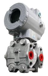
The electronic resonance circuit reads capacitance variation between the moving and fixed plates. The CPU conditions the measurement and communicates according to protocol. As there is no A/D conversion, errors and drifts during conversions are eliminated. A temperature sensor provides temperature compensations, which combined with the sensor precision, results in high accuracy and rangeability for the LD300 Series.
